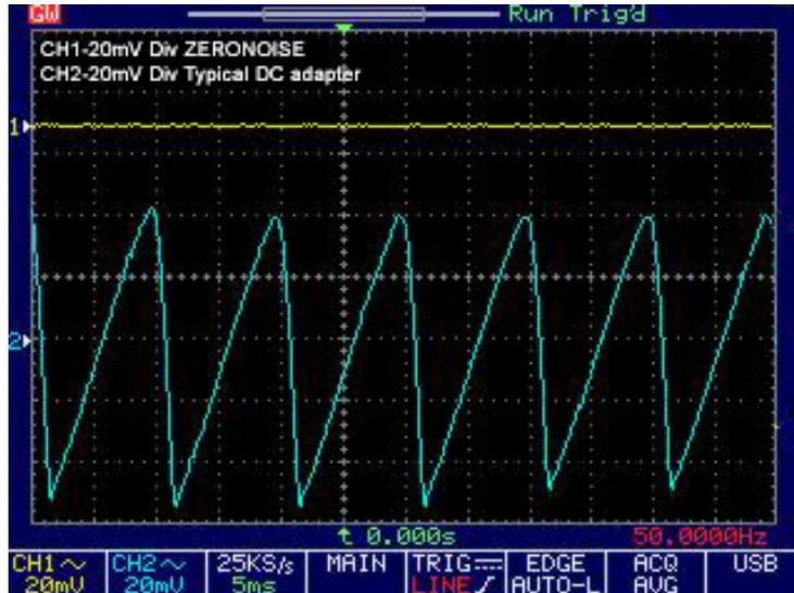
In the diagram (a) you can see the differences from a typical AC to DC adapter against **ZeroNoise Road**. The graphic shows that the DC output from the standard adapter introduces much more ripple noise into the signal as compared to the clean power produced by **ZeroNoise Road**.
